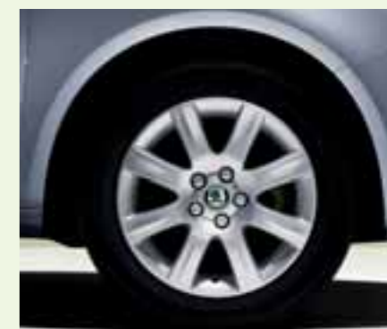
6.0J x 15" Line alloy wheels for 195/55 R15 tyres.
