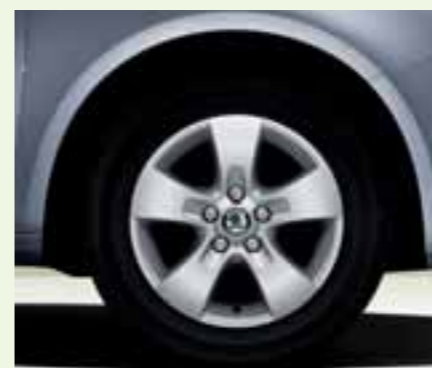
6.0J x 14" Atik alloy wheels for 185/60 R14 tyres.
