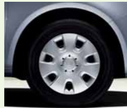
5.0J x 14" steel wheels for 165/70 R14 tyres with Draco hub covers.
